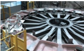
Image 1 Scrap aluminium is sent for recycling Image 2 Carousel for pouring off aluminium
